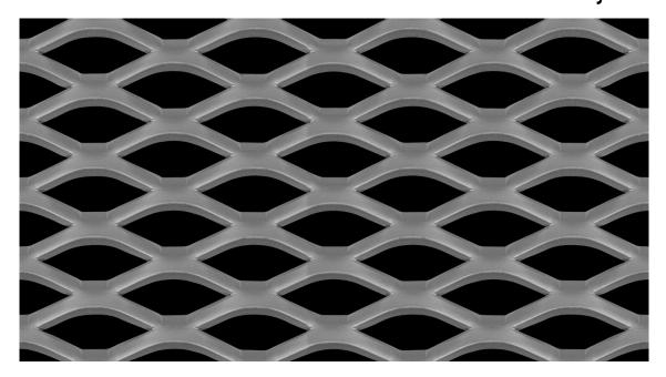
LW Pitch:38.10mmStrand Width:4.75mmSW Pitch:16.93mmThickness:3.00mmWeight:13.20 kg / m2Open Area:44%
